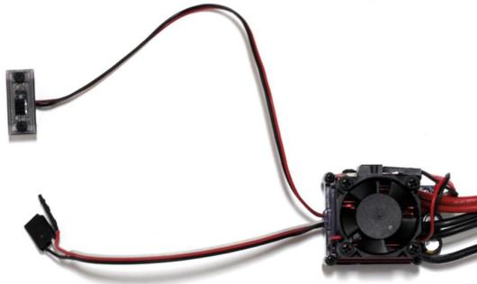
B. This photo shows the BEC and battery plugs. The ESC is equipped with a standard Tamiya plug. This should make it an easy plug and play for your battery connections. (changing the plug may void your warranty)
