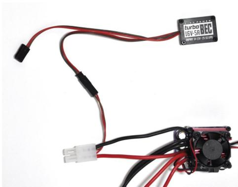
C. The motor wires are shown in this photo. Again the dual motor ESC was used for this manual. The single motor ESC will only have the two motor wires. One black and one red. The dual motor has two black and two red.
