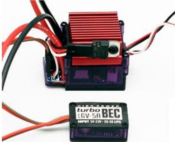
**The Outcry ESC is designed for Radio Control Crawler or Scaler use. The ESC is has a built in non-adjustable drag break. The ESC comes with a BEC (battery eliminator circuit). This allows you to get full power to the other electronics in your setup.**
